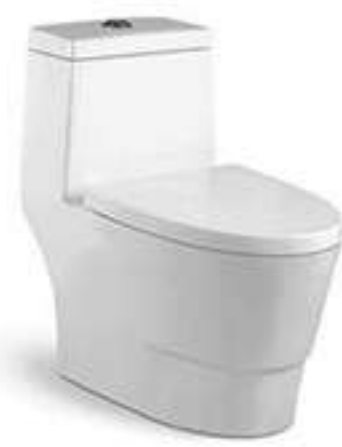
1545-2855 Washdown / Siphonic one-piece toilet Size: 680x390x710mm Washdown: S-trap: 250mm Roughing-in Siphonic: S-trap: 250/300mm Roughing-in P-trap: 180mm Roughing-in
