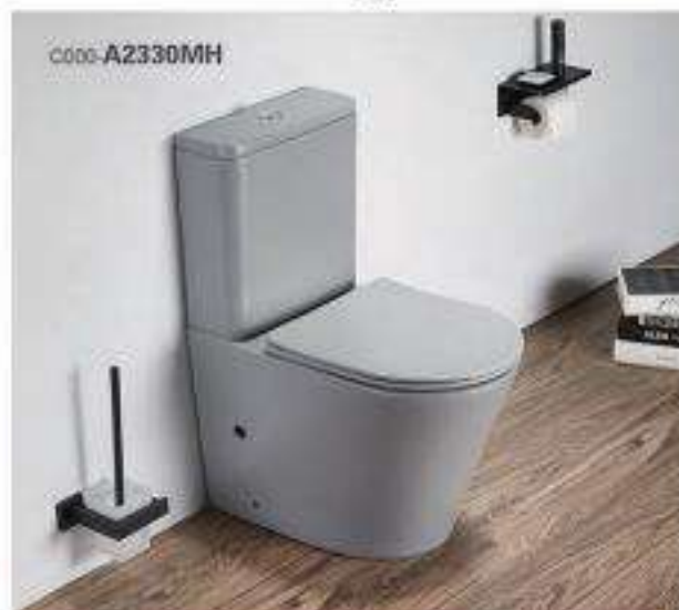
C000-A2330 Washdown two-piece toilet Size: 610x370x760mm S-trap: 250mm Rounding-in P-trap: 180mm Rounding-in
