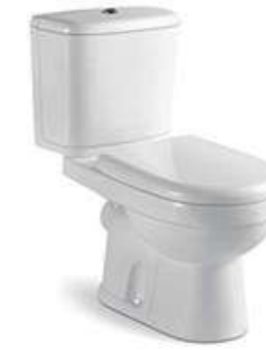
1560-2967 Washdown two-piece toilet Size: 710x410x750mm S-trap: 250mm Roughing-in P-trap: 180mm Roughing-in
