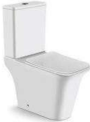
C000-2973 Washdown two-piece toilet Size: 660x350x820mm S-trap: 250mm Routing-in P-trap: 180mm Routing-in
