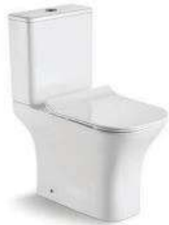
C000-2971 Washdown two-piece toilet Size: 600x340x770mm S-trap: 250mm Routing-in P-trap: 180mm Routing-in
