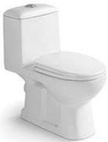
1549-2951 Washdown one-piece toilet Size: 660x350x680mm S-trap: 250mm Roughing-in P-trap: 180mm Roughing-in
