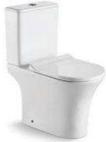
C000-2970 Washdown two-piece toilet Size: 650x340x770mm S-trap: 250mm Routing-in P-trap: 180mm Routing-in
